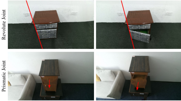
Figure 8. Visualization of the revolute axis and prismatic joint of articulated objects.
