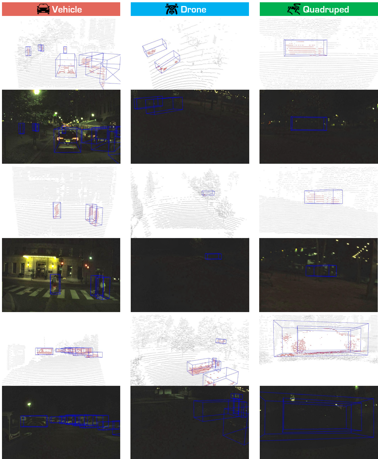
Figure I. Examples of 3D object detection annotations from 3D (LiDAR point cloud) and 2D (RGB image) in our Pi3DET dataset. We provide data from three robot platforms : Vehicle , Drone , and Quadruped . Best viewed in colors.
