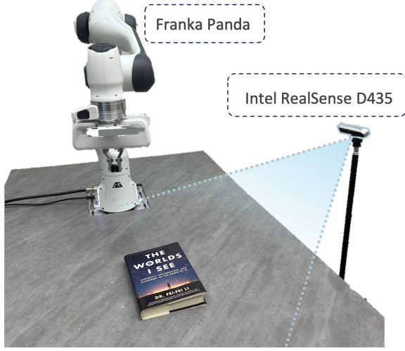
Figure 7. Real-world Experiment Setup
