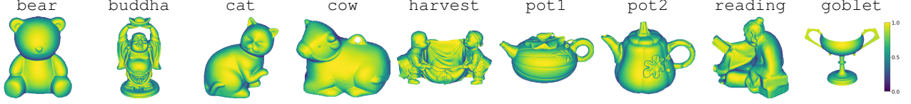
Figure 8. Visualization of the terms |n_a^T \tau_a| , DiLiGenT dataset [31]. The terms encode the degree of collinearity between the surface normals and the ray direction vectors. Low values are attained at pixels where the ray direction vector is perpendicular to the surface normal, a necessary condition for the corresponding point to lie on the object boundary.
