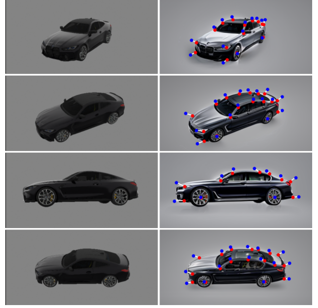
Figure 8. Example of the point translation function for the vehicle domain. In this case. The dimensions of the reference object (left column) are width_r = 1.89m, length_r = 4.79m, height_r = 1.39m and the target dimensions of the vehicle are width = 1.95m, length = 5.391m, height = 1.544m . For \delta length . This results in the points marking the front lights and bumpers being moved by +0.3005m along the y-axis and the points for the rear lights and bumpers by -0.3005m . The change in width of \delta width = 0.06m leads to all points on the left half of the car being moved by +0.03m along the x-axis and all points on the right by -0.03m . For \delta height = 0.154m , all points except for the wheel centers and the bumpers are moved for +0.154m in z. Depending on the viewpoint, the visible geometry points are affected by the point translation function.
