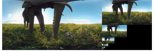
Figure 3. Mipmapped image with 8 mipmap levels. For each mipmap level, the original image is downsampled by a factor of 2 including Gaussian pre-filtering for antialiasing.
