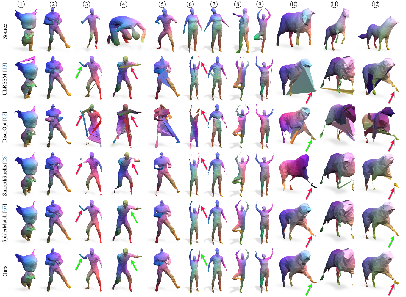
Figure A.7. Additional qualitative shape matching results on datasets DT4D-H (columns ①-⑤), FAUST (columns ⑥-⑨), and SMAL (columns ⑩-⑫). Columns ①, ③, ⑤, ⑥, ⑨, ⑩ are also shown in the main paper and are repeated here for comparison with methods DiscrOpt [62] and SmoothShells [28]. All matchings are visualised by transferring colour and triangulation from source to target shape. In column ⑫, we can see a failure mode of ours very likely caused by the fact that our solution space still contains matchings which allow for inside out flips (one side of the leg is matched to the other side of the leg).
