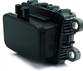
Figure 1. Experimental FWL Sensor. We adapt a MicroVision MOVIA™ L Sensor [17] to output full waveform data.
