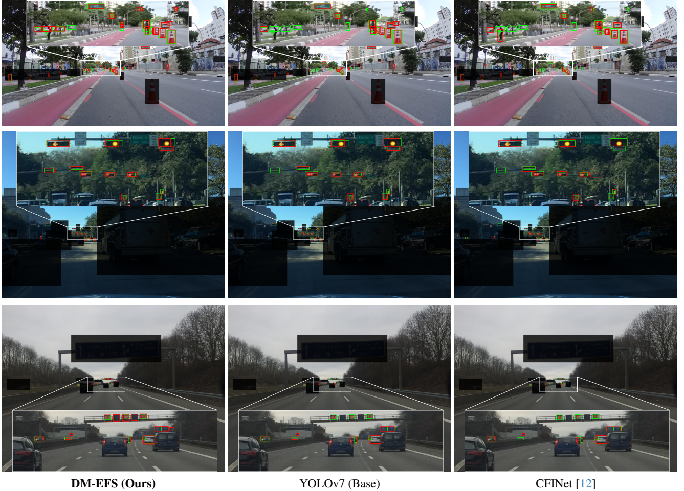
Figure 1. Results on the SODA-D dataset. We can see that our DM-EFS outperforms both the YOLOv7 base model and recent SOD method CFNet. Note, green and red boxes are ground-truths and predictions respectively, and ‘ignore’ regions are masked out. All the results are shown without class labels for ease in visualization and performance comparisons.
