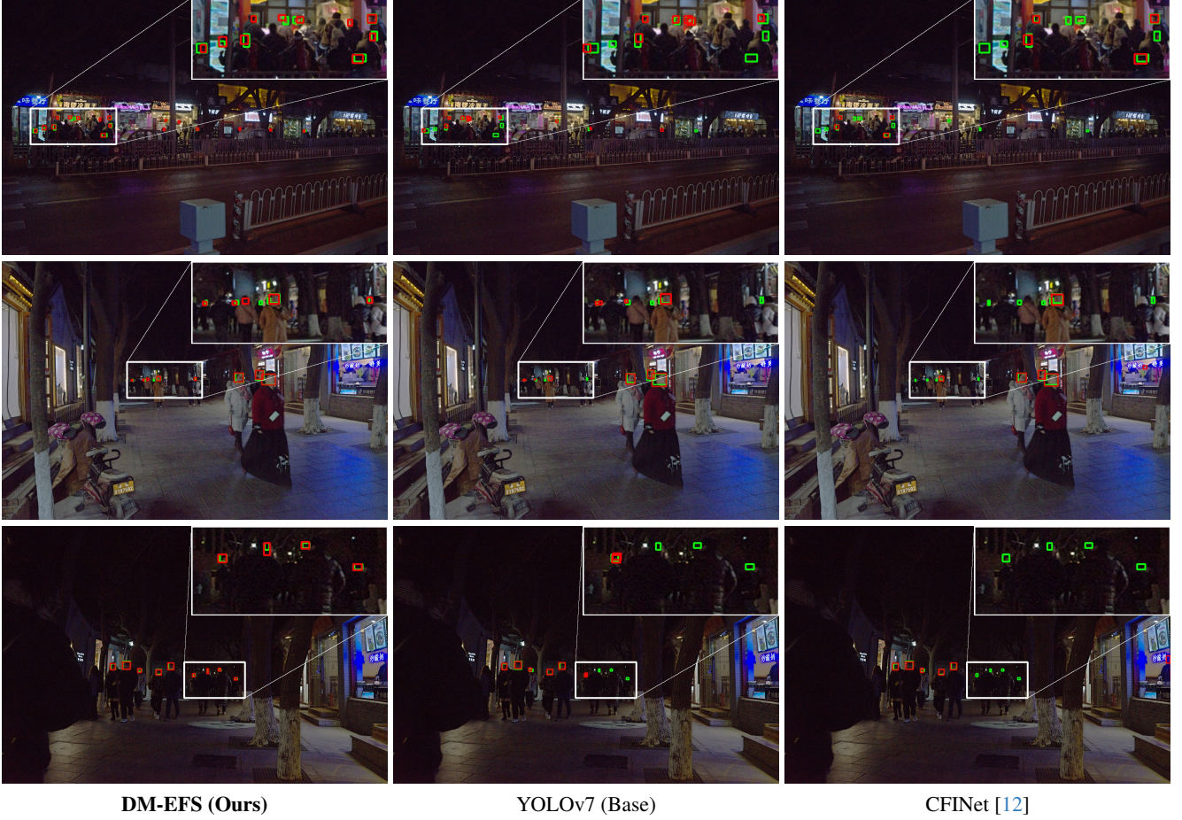
Figure 7. Results on the DarkFace dataset. We can see that our DM-EFS outperforms both the YOLOv7 base model and recent SOD method CFINet in detecting small faces robustly. Note, green and red boxes are ground-truths and predictions respectively. The results are for 640 \times 640 images but are shown on original images for ease in visualization.
