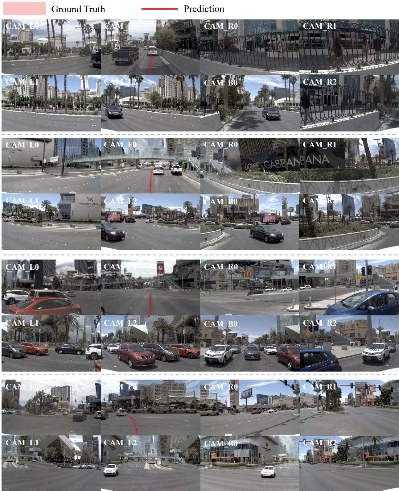
Figure 7. Qualitative results of end-to-end driving on NAVSIM test set. DriveX successfully handles challenging scenarios including breaking, lane changing, intersection negotiation, and turning maneuvers.
