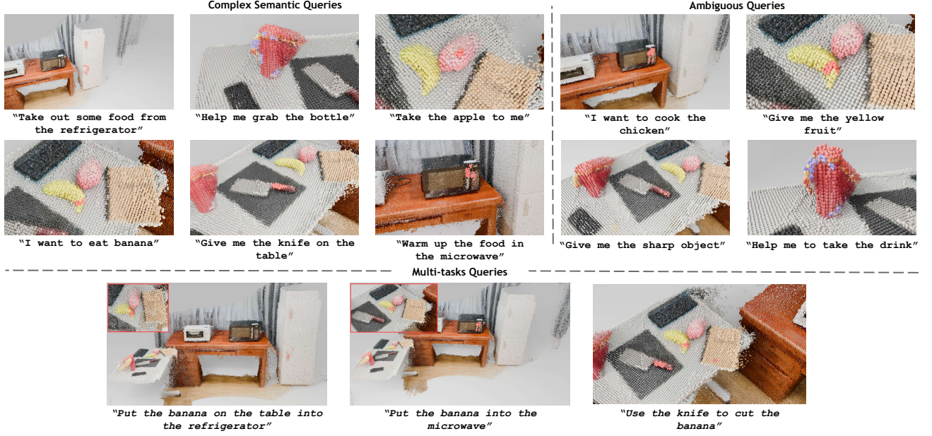
Figure 1. Experimental results of our framework detecting affordance locations in real-world scenes based on user commands. This demonstrates the superior affordance detection ability of the OVA-Fields across various objects and tasks. The OVA-Fields also handles ambiguous queries and multi-tasks queries effectively, accurately identifying relevant affordance locations even when user instructions are ambiguous
