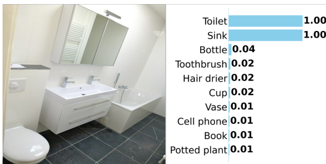
Figure 2. Inference of ResNet-50 [6] model trained with our AEVLP method on images from COCO [11] test dataset.
