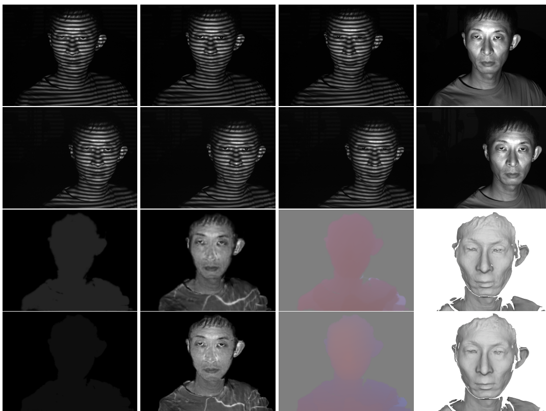
Figure 8. Additional results of the real-world experiment. Captured images from camera 1 and camera 2 under uniform lighting and three phase-shifting patterns (first and second rows), and residual (brightness \times 5 ), reflectance, and displacement field projected to the camera 1 view and the reconstructed 3D shape after 10,000 and 20,000 training iterations (third and fourth rows).
