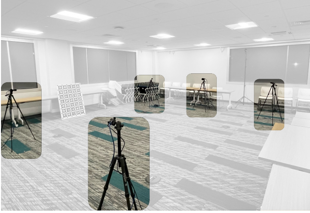
Figure 14. BEAHM collection setup. 4 high speed cameras for gt are placed at 4 corners and a beam splitter is placed at one side to capture human in the middle of the room. The space of acting zone is 1.5\text{m} \times 2\text{m} .
