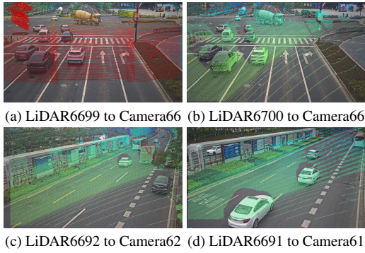
Figure 13. Roadside LiDAR/Camera calibration results. The various point color represent the relative distance to the origin.
