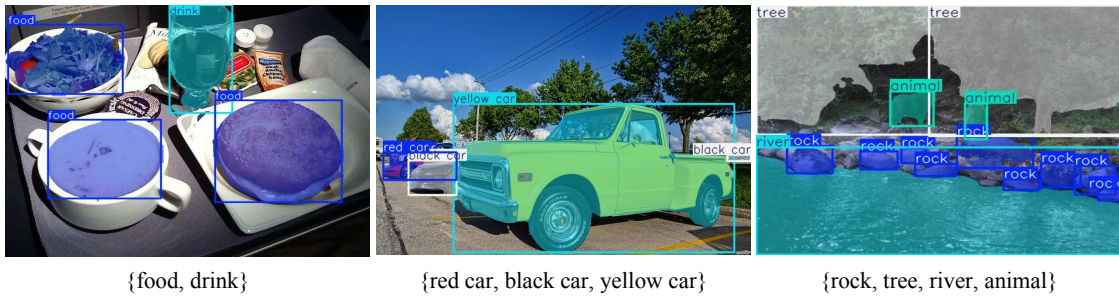
Figure 3. Prompt with customized texts. YOLOE adapts to both generic and specific text prompts for flexible usage.
