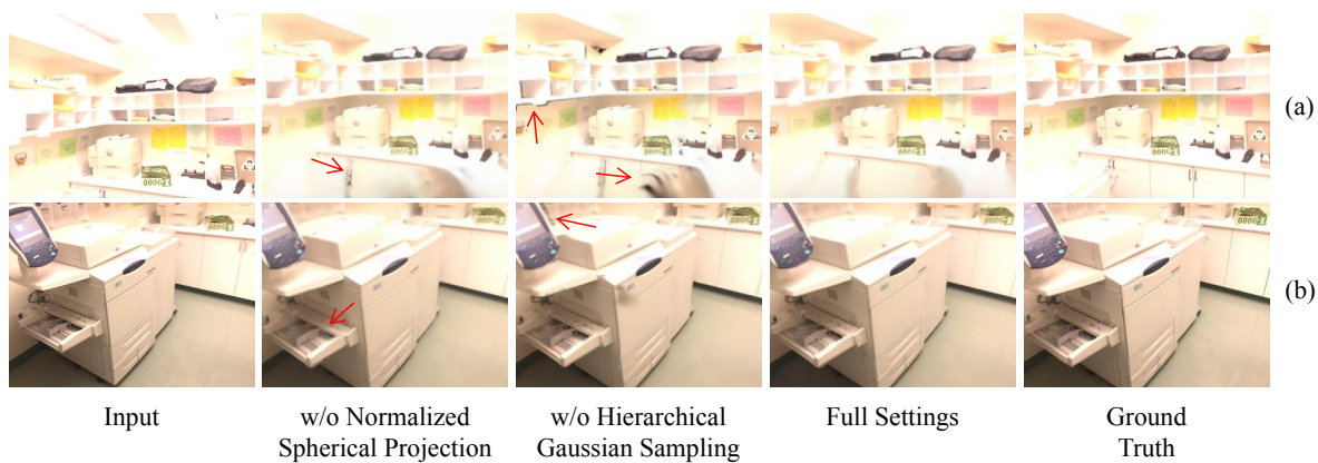
Figure 3. Ablations on BundleFusion (val). Without Normalized Spherical Projection, our model fails to reconstruct outside the input FOV, leading to ghosting artifacts. Without Hierarchical Gaussian Sampling, there will be ripple artifacts and holes in the rendered novel views.
