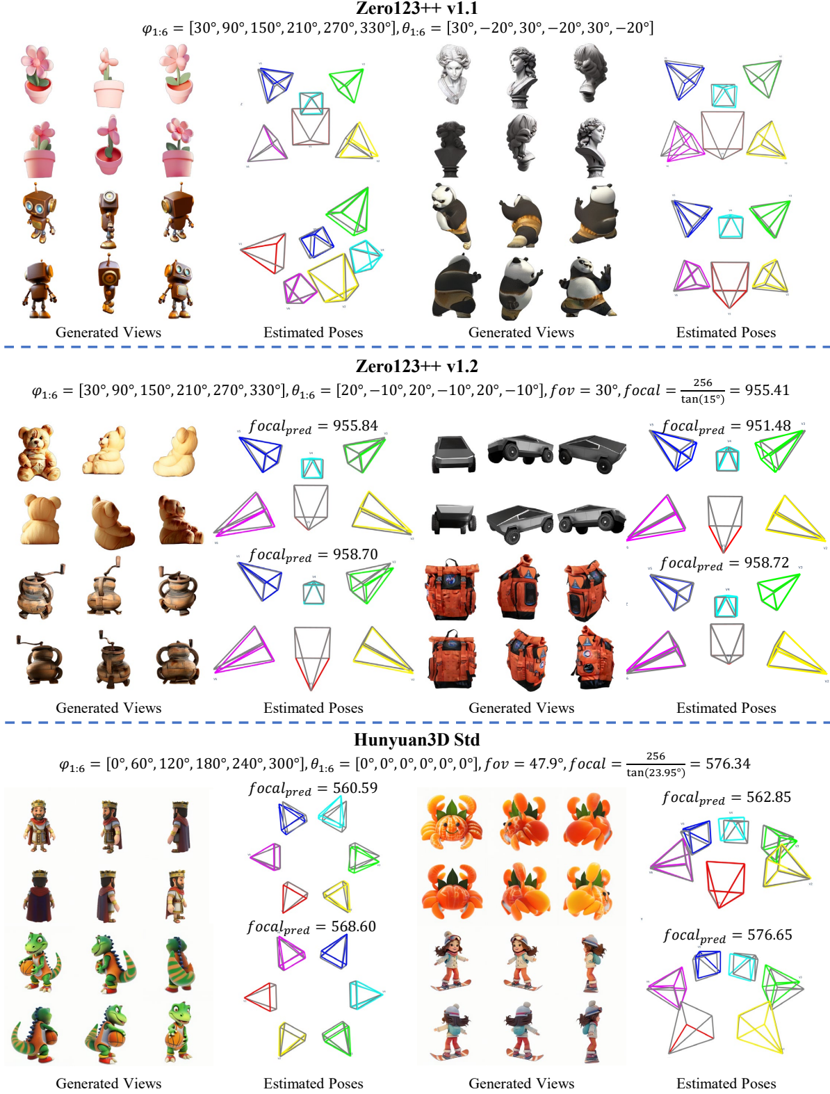
Figure 6. Camera Pose Estimation on Images Generated by Multi-view Diffusion Models. FreeSplatter can faithfully recover the pre-defined camera poses of different multi-view diffusion models. We visualize the predefined camera poses of diffusion models and the estimated poses with gray and colorful pyramids, respectively. \varphi and \theta denote the predefined azimuth and elevation angles, respectively. For Zero123++ v1.2 and Hunyuan3D Std which generate images at predefined fixed focal lengths, we mark the predicted focal lengths (in pixel units) too.
