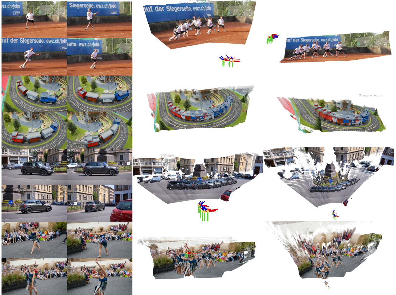
Figure 4. Visual results on DAVIS [23] with camera poses estimated from the output point maps. We concatenate 8 aligned point maps from the original point map sequence for visualization.
