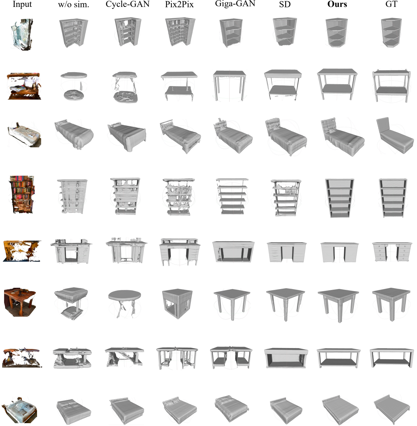
Figure I. Qualitative comparison on 3D instance reconstruction, using LASA [4] training data mixed with simulated data generated by different methods. “Rand.” means random perturbation. “w/o sim.” denotes using LASA training data without simulated data.
