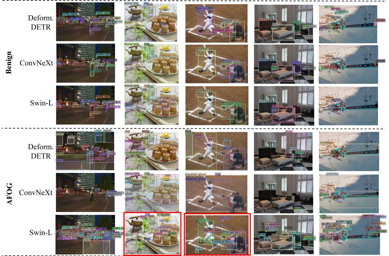
Figure 13. Comparison of Benign and AFOG-disrupted predictions on five example images with Deformable-DETR, ConvNeXt, and Swin-L. AFOG exhibits widely varying behavior for different models on the same image, such as against image three (Rows 4-6, Col. 3). We also indicate two instances where AFOG failed to disrupt Swin-L’s performance, highlighted in red.
