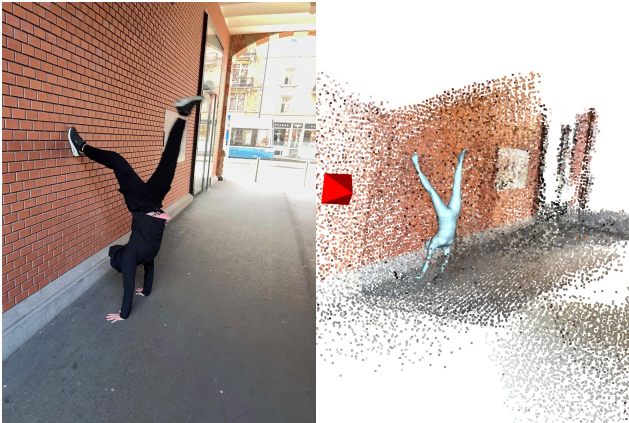
Figure 13. Adaptive contact joint identification for a handstand example, where our method correctly identifies the hands as the contact points, ensuring robust scale calibration for unusual postures where the feet are not the real contacts.
