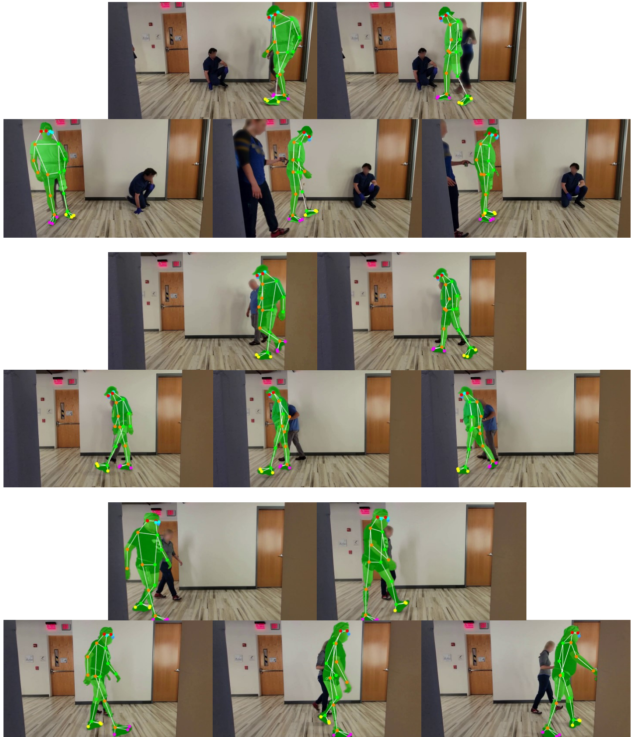
Figure 4. Videos and corresponding annotations captured at sagittal view outside the parallel bar. Subjects 1, 2, and 4 walking alongside the hallway with mechanical knees, accompanied by the healthcare staff.
