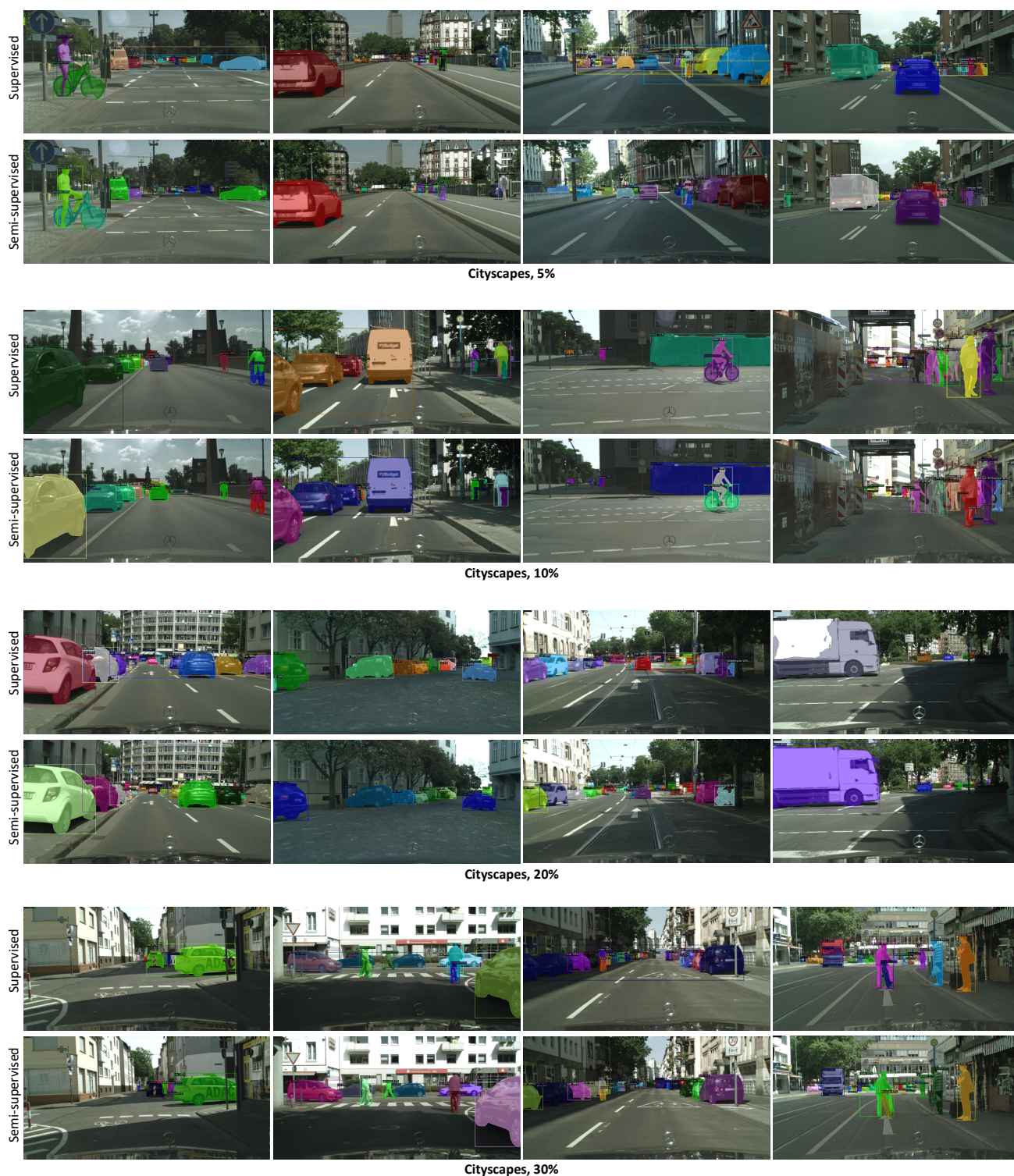
Figure A.1. Qualitative results on Cityscapes under different labeled data settings. Predictions from supervised training (top) and our semi-supervised approach (bottom) across different labeled data settings. "Supervised" refers to the pretrained teacher network, while "semi-supervised" denotes the student model trained jointly on both labeled and unlabeled data.
