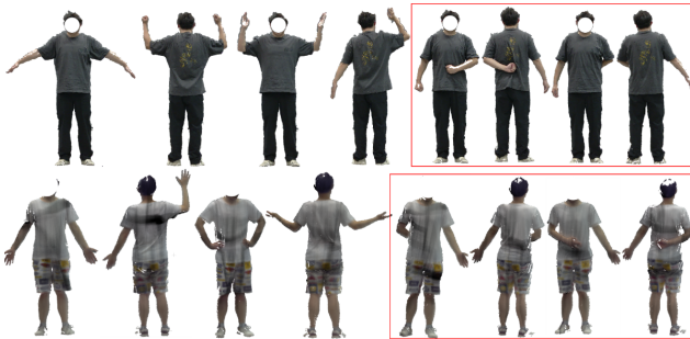
Figure 13. The upper eight point clouds were captured with the Orbbec Astra 2, and the lower eight with the CR-Scan Otter 3D Scanner. The red rectangles indicate designed postures.
