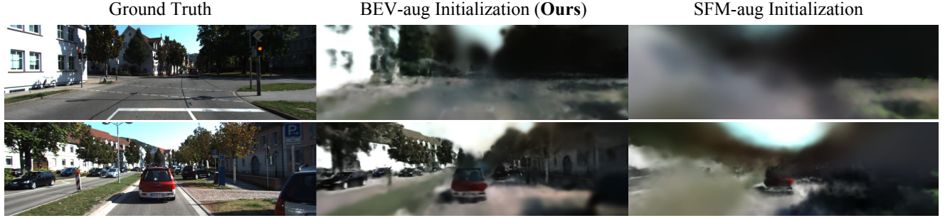
Figure 8. Visualization Results of BEV-aug Initialization and SfM-aug Initialization. The BEV-aug initialization approach provides reliable initialization for tall structures that are inadequately captured by LiDAR sensors. In contrast, the SfM-aug initialization method often suffers from inaccurate initialization due to misalignment between the SfM-estimated point clouds and the LiDAR data.
