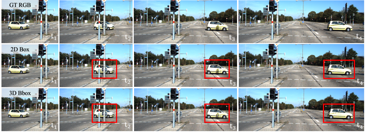
Figure 9. Qualitative Comparison with Different Decomposition Methods. Decomposing the object and static elements with 2D boxes and modeling object motion trajectories with NeuralODE produce competitive results to precise 3D bounding boxes.
