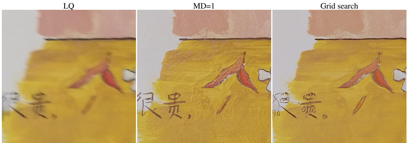
Figure 7. Demonstration of the occasional discrepancy between human preference and non-reference metric. The grid search result (right) removes motion blur from the LQ (left), but also impacts fidelity. However, by manually setting the weight for motion deblur (MD) to 1 and the rest to zero, a visually better result can be obtained (middle). This is an example where non-reference metric is not fully aligned with human preference.
