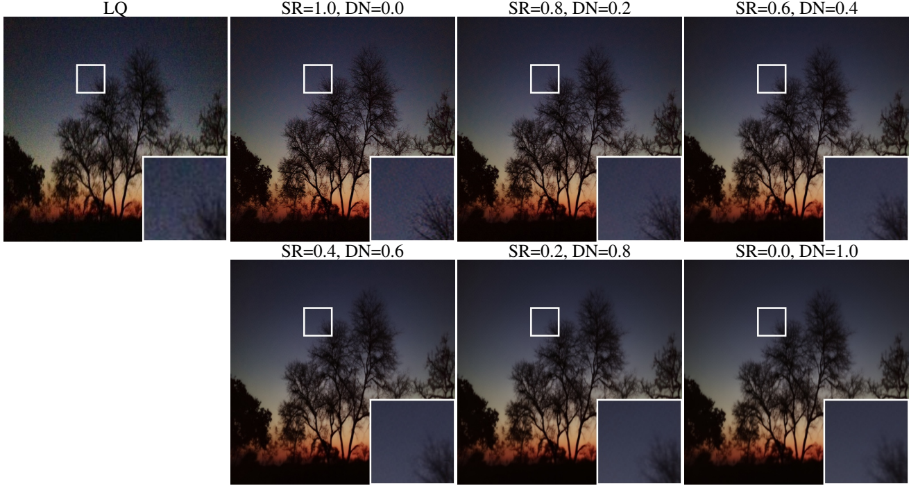
Figure 4. Qualitative demonstration on combination weight sensitivity. In this example, we adjust the weights for super resolution (SR) and denoise (DN), and keep the rest weights to zero. As shown from the images, the SR=1 case can improve the details to the tree, but does not remove all noise. In contrast, the DN=1 case can remove the noise, but not improve the details of the tree. By trading off the two weights, we can observe a smooth trade-off between the two effects. Zoom in for image details.
