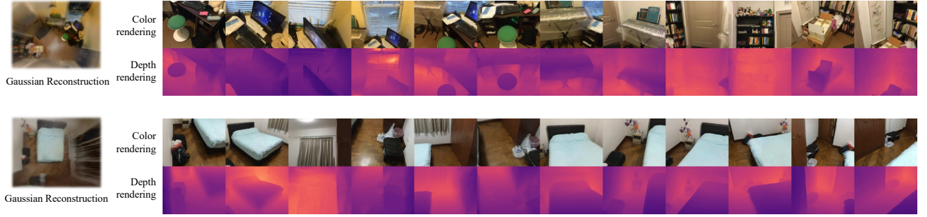
Figure 5. Zero-shot reconstruction results on ScanNetv2 from Long-LRM (2D GS ver.). We render both RGB images and depth maps from the predicted 2D Gaussians. The depth maps exhibit fine object details, demonstrating Long-LRM’s capability for instant geometry reconstruction on complicated novel scenes.
