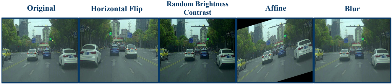
Figure 1. A visualization of the various methods used to augment images. The first image from the left is unaltered, the second is horizontally flipped, the third's contrast and brightness have been altered, the fourth has an affine transformation, and the last has been blurred. The hyperparameters for these augmentations are mentioned in Table 2 .
