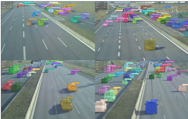
Figure 6. Visualization of labeled sequence S03. A vehicle is not maintaining safety distance to the leading vehicle. It changes the lane to the right and hits another two vehicles. One of them is full 360-degree spin.
