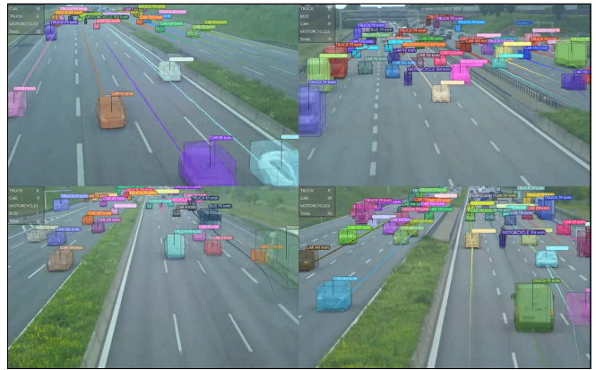
Figure 14. Visualization of labeled sequence S10. A truck is changing lanes and rams a passenger vehicle from the side. It is spinning 180-degree in one direction and then in the other.
