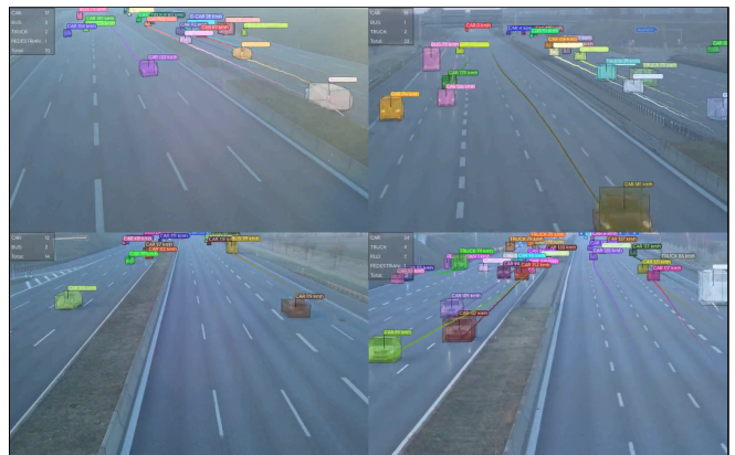
Figure 16. Visualization of labeled sequence S12. A vehicle is speeding and crashes into a van that has a breakdown on the left lane.
