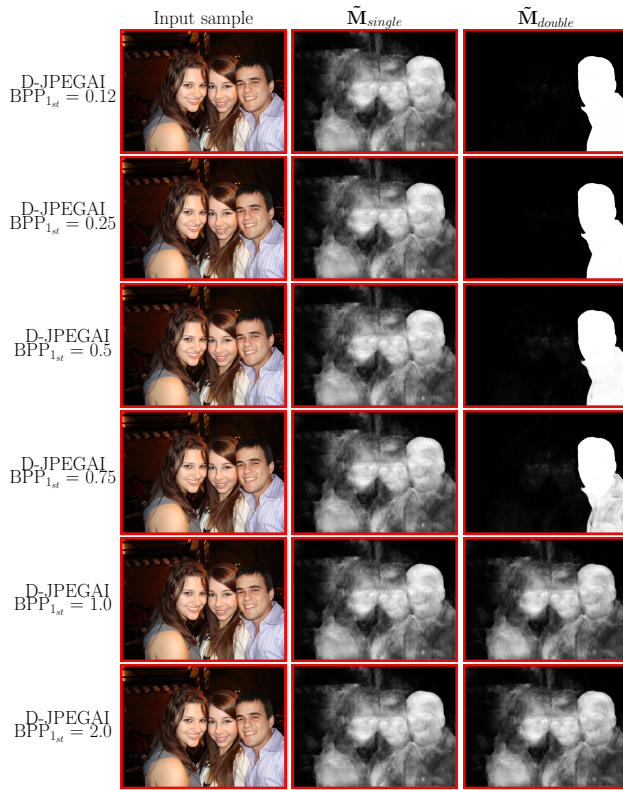
Figure 20. Output of MMFusion for DSO-1 double JPEG AI compressed images. The second compression stage is executed with BPP equal to 2.0. The first compression stage BPP value varies from 0.12 to 2.0 from top to bottom.
