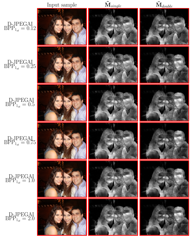
Figure 19. Output of MMFusion for DSO-1 double JPEG AI compressed images. The second compression stage is executed with BPP equal to 0.12. The first compression stage BPP value varies from 0.12 to 2.0 from top to bottom.
