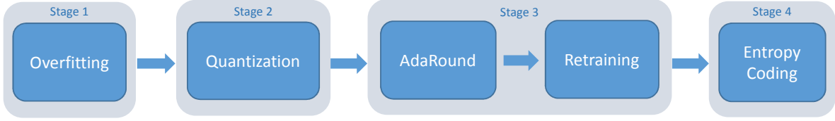
(a) Overview of INR-based compression pipeline proposed by Y. Strümpfer et al. [49]. The basic compression pipeline comprises image overfitting, quantization of the neural network, AdaRound, retraining, and lossless entropy coding (e.g. binarized arithmetic coding).
