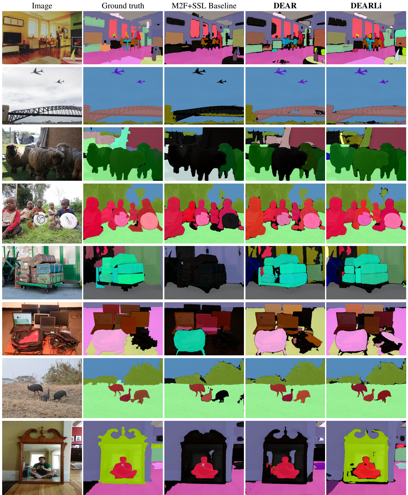
Figure 8. Panoptic predictions of the baseline M2F+SSL CN-B-L2B ( cf. Tab. 1 in the main manuscript), DEAR, and DEARLi on few examples from the COCO-Panoptic val. All models are trained on the COCO-Panoptic 1/512 data partition ( i.e. , only 232 labeled images).
