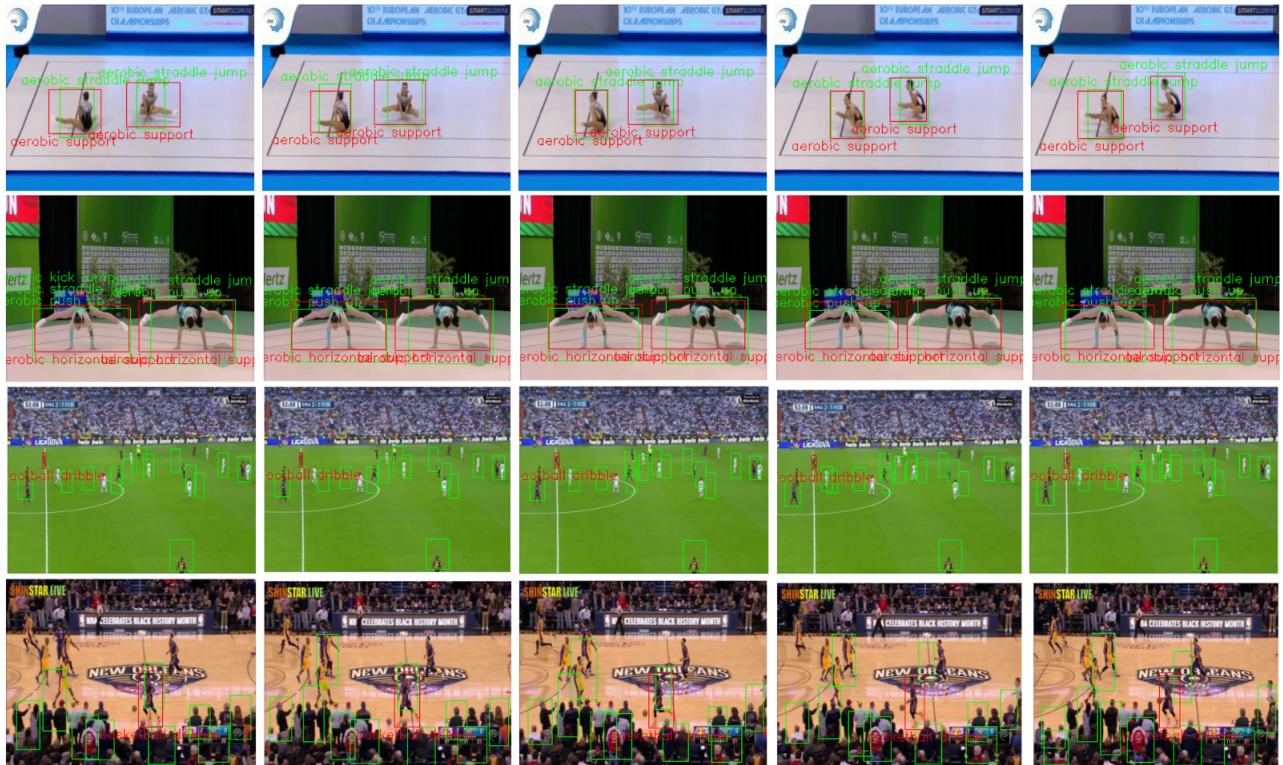
Figure 6. Additional Visualizations from MultiSports : Our model is able to detect the sport, but not the associated fine-grained action in each sport. In addition, our model fails at detecting long-range humans. The predicted actions in row 3 (football) and row 4 (basketball) are removed for cleaner visualizations since all the fine-grained actions in both sports are detected as positive by our model.
