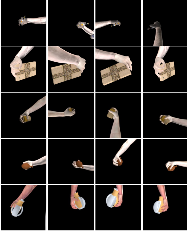
Figure 1. Example from the Multi-View ObMan synthetic dataset: Each row represents a single hand-object scene and columns is a different view of the same hand-object. Hand-objects are rendered on a black background, black background is acceptable as pointmap estimation network is trained with only hand-object masked pixels.
