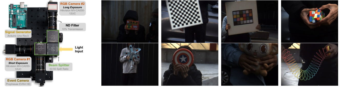
Figure 1. Left: Our hybrid camera system, which consists of three cameras: an event camera, and two RGB cameras with short and long exposure time, respectively. Right: Some scenes in the EvRGB-Deblur dataset.
