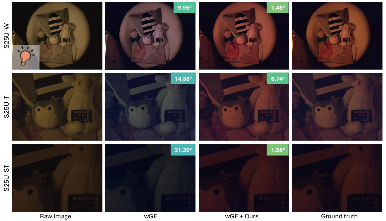
Figure 5. Qualitative results. Shown is an indoor scene illuminated by an orange LED light, captured by the S25U wide, telephoto, and super-telephoto sensors, white-balanced using wGE [3] predicted illuminant, wGE corrected with our mapping, and the ground truth aesthetically-preferred illuminant.
