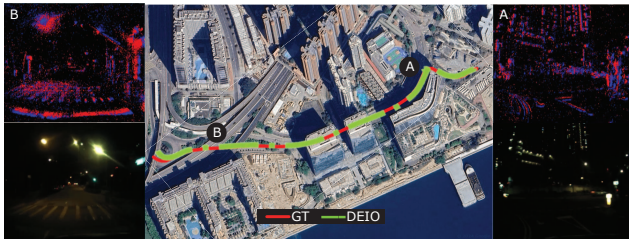
Figure 3. The estimated trajectory of our DEIO in the night driving scenarios [3] and its comparison against the GNSS-INS-RTK as ground truth. The image view is for visualization only.
