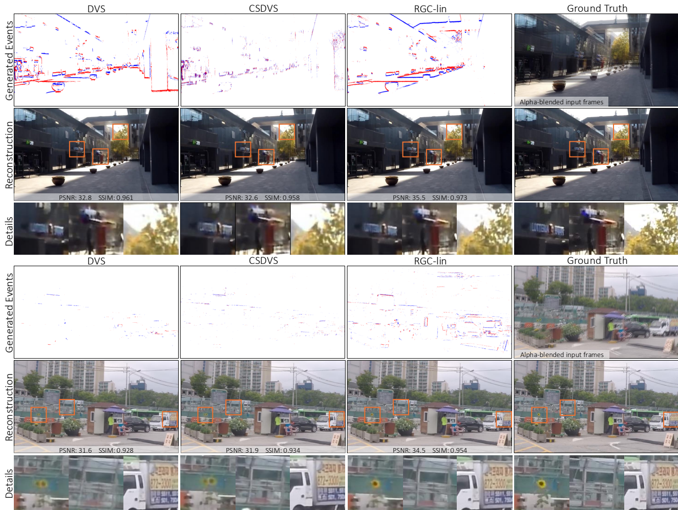
Figure 3. Video Interpolation Qualitative Results. For each scene, we compare the reconstructions of the middle frame in the sequence for DVS, CSDVS, and RGC-lin. The top row shows the generated events, binned into the corresponding middle time bin, the second is the predicted image and the bottom row shows zoom-ins. The right-most column shows the start and end frames, alpha-blended, ground truth frame, and zoom-ins. PSNR(↑) and SSIM(↑) metrics are shown for each reconstruction.
