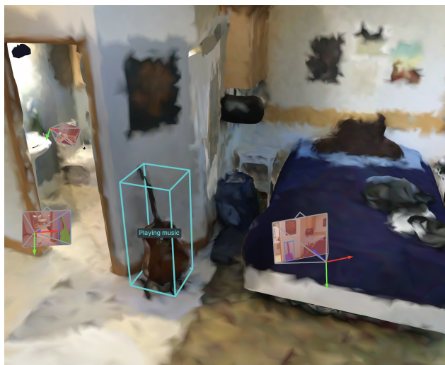
Figure 1. Open-vocabulary 3D Object Detection. Our method takes as input a sparse collection of posed RGB images together with a query text prompt. The outputs are 3D bounding boxes corresponding to the prompt. In the figure we include the ground-truth mesh for visualization purposes only.
