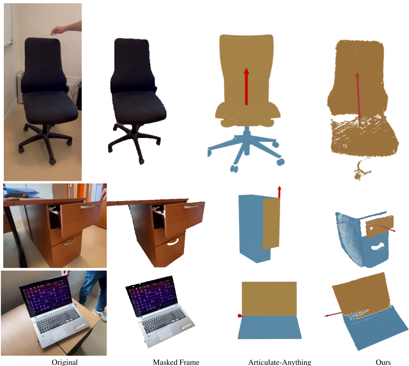
Figure 3. Qualitative results on the chair, storage, and laptop objects from the real objects dataset. We show joint estimation, mesh reconstruction and part segmentation results. As shown in the figures, Articulate-Anything retrieves an incorrect mesh for the storage object and inaccurately predicts both the joint type and axis. Similarly, it predicts an incorrect joint axis for the laptop and an incorrect motion direction for the chair. It is important to note that Articulate-Anything does not perform geometry reconstruction; instead, it retrieves meshes from a predefined database. Therefore, our objective here is to evaluate its performance in mesh retrieval and joint prediction. Refer to the supplementary video for the animated mesh results.
