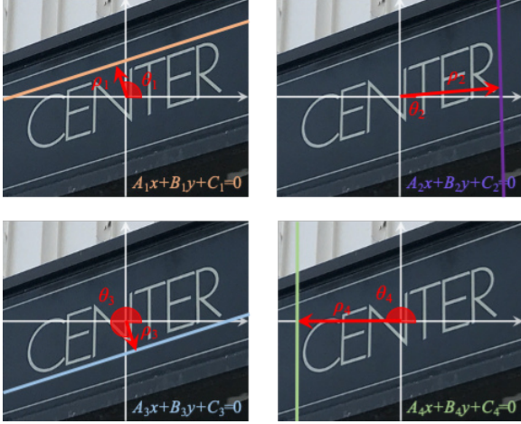
Figure 3. The visualization of four parameterized line equations with cartesian coordinates (orange, purple, blue and green) and polar coordinates (red).
