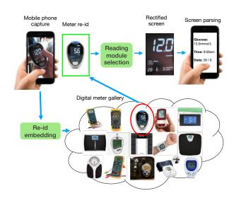
Figure 1. Recognition and screen reading on mobile phone. Our system can both recognise and parse the screen of a digital meter at near 100% read accuracy. The system is trainable using a single human labelled image consisting of a binary mask indicating screen and background pixels, and the four corner coordinates of the screen, see Figure 2. For meter recognition the system matches a deep re-id embedding to the best matching meter in a gallery of collected digital meters.
