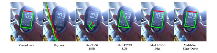
Figure 8. **Qualitative comparisons.** Examples of screen detections for blood glucose meter, quadrangles are shown as green polygons with the red edge indicating screen top. Comparison shown against baselines.
