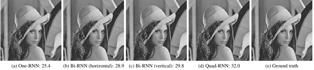
Figure 8: Inpainting with different directional RNNs and corresponding PSNR. (a) Single-directional RNN, scanning from left to right. (b) Bi-directional RNNs with horizontal scans. (c) Bi-directional RNNs with vertical scans. (d) Quad-directional RNNs with horizontal and vertical scans.
