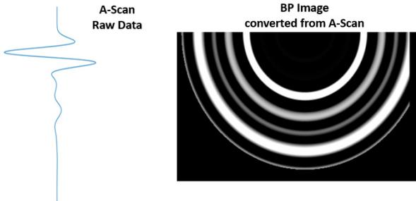
Figure 4. The implementation of BP algorithm which would convert the A-scan raw data into several semi-spheres.
