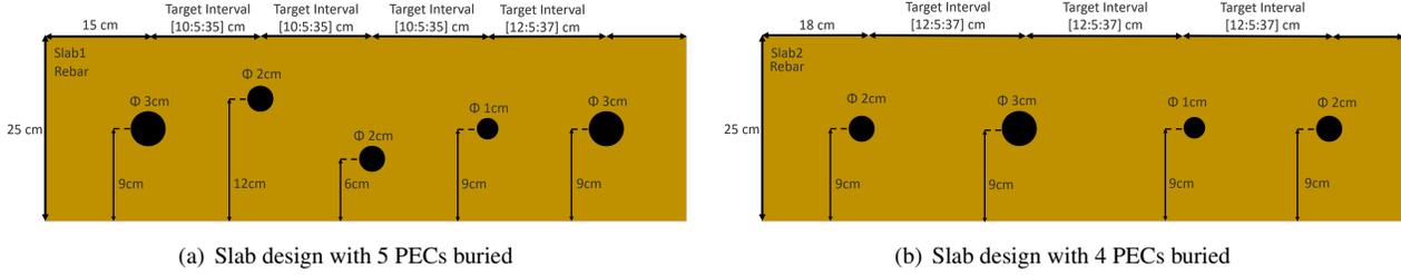
Figure 3. Slab design with different number of PECs and different PEC intervals.
