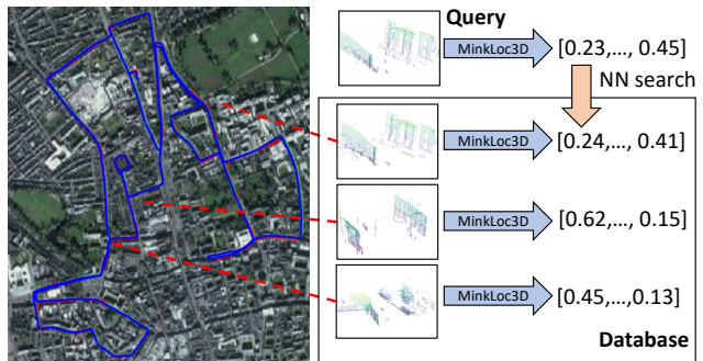
Figure 1. Point cloud-based place recognition. MinkLoc3D computes a global descriptor of a query point cloud. Localization is performed by searching the database for geo-tagged point clouds with closest descriptors.
