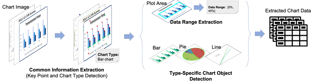
Figure 2: ChartOCR framework outline. There are three major steps: common information extraction, data range extraction and type specific chart object detection. Common information extraction aims to detect the keypoints and the chart type. Data range extraction infers the range of the data that the chart represents. Type specific detection focuses on extracting the chart objects (eg. bars, lines and etc).
