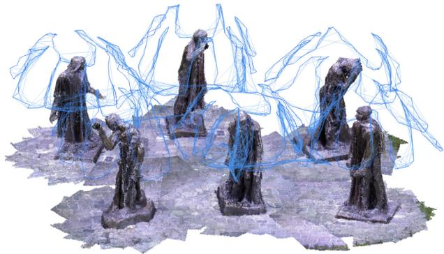
Figure 1: Camera trajectory, loop closures and 3D reconstruction of the Burghers dataset [25] using our algorithm.
