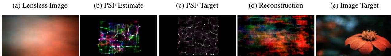
Figure 6: **Blind Deconvolution Reconstruction:** We display results from a blind deconvolution method in [31], which struggles to estimate the PSF or the image correctly. Blind deconvolution methods traditionally work well for estimating motion blur or more structured optical blur PSFs as opposed to the randomness of a diffusion PSF.
