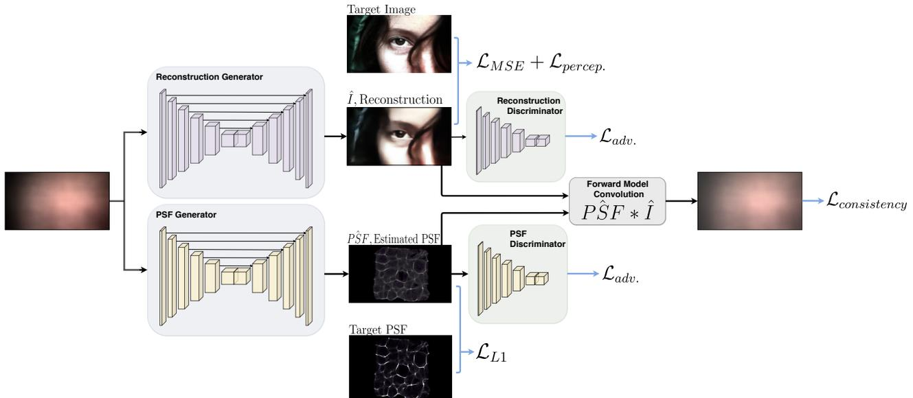
Figure 1: **Network Architecture:** Our lensless image reconstruction pipeline consisting of generative adversarial networks for image reconstruction and point spread function (PSF) estimation. In addition to regular and adversarial loss functions, a perceptual loss and a self-supervised consistency loss with respect to the forward imaging model is incorporated.
