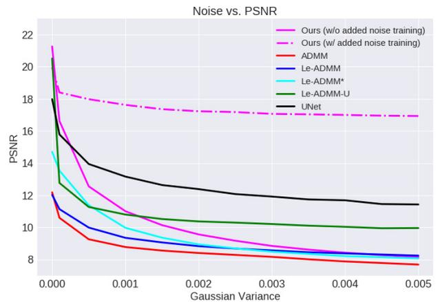
Figure 4: **Noise:** Ablative study of model performance with respect to additive Gaussian noise. Notice how even an extremely small amount of noise ( $\sigma^2 = 0.005$ ) results in degradation of performance for all methods. However, specifically training our model with noise results in more robust performance.
