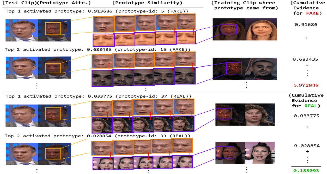
Figure 3. The reasoning process of the DPNet. The prediction for video clip is based on the similarity comparison between the latent input representations against the learned prototypes. The network tries to find evidence for manipulated/genuine by looking at which spatial/temporal patch that was mostly activated by the dynamic prototypes. Similarity scores between class-specific prototypes are summed.
